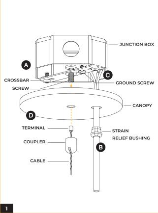
(A) Secure the crossbar to the junction box (by others) designed to support the weight of the fixture.
