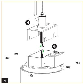
(E) Make electric connection inside the wiring box.
