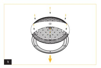
Remove six screws on the top of the fixture to release the bottom cover plate.
