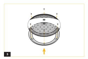
Reattach the bottom cover plate, and then tighten the six screws on the top of the fixture.
