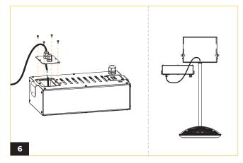
Unscrew the DC junction box and loosen the cable clamp. Insert the FC wire through the cable clamp and connect them to the wires in the junction box. Refer to wiring diagram for detailed explanation of wiring diagram.
