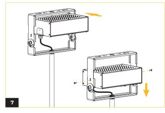
Slip the power box hook fastener over the lock-in grooves allocated and fasten screws on either side to keep the power box in place.
