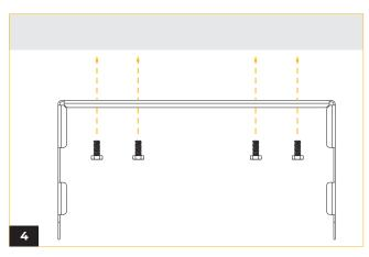
Fasten the top bracket on the desired location on the ceiling.
