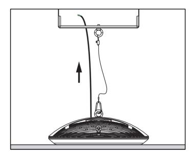
**Step 3**Attach the fixture cables through the lower bracket.
