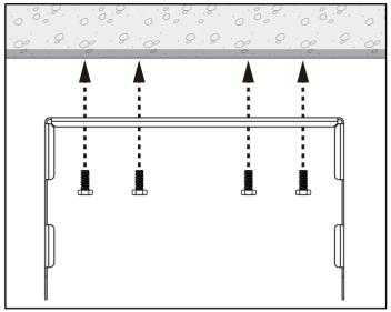
**Step 4**Fasten the top bracket on the desired location on the ceiling.
