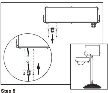
Open the DC Junction box and connect cables. Refer to wiring diagram section.  $\,$
