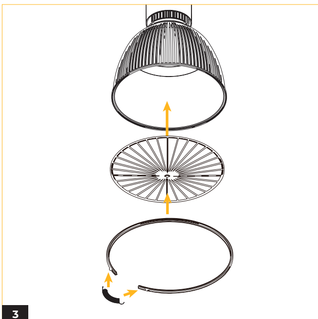
Cover the shroud with the conical lens plate and fasten it in place.
