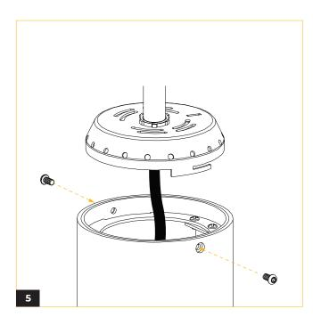
Replace lid and secure two Allen screws.
