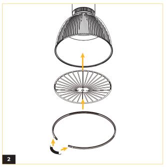
When specifying the conical lens accessory. Cover the shroud with the conical lens plate and fasten in place using the provided metal band.
