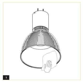
Clean the interior and exterior surface using a soft rag with
