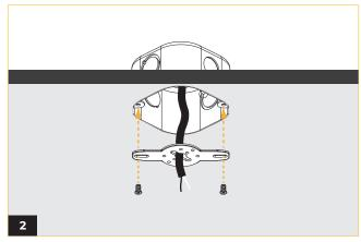
Secure the crossbar to the junction box (supplied by others), using two Phillips screws.
