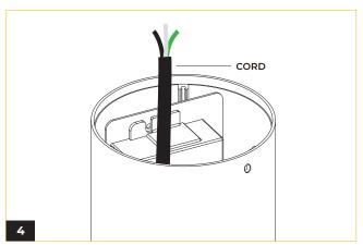
Make electrical connections between the junction box and the fixture with UL listed connectors or wire nuts (supplied by others). Refer to the wiring diagram below.
