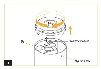
Loosen two screws on the side of the fixture. Twist and lift up the lid from the cylinder. Unhook the safety wire from the cylinder to detach the lid.
