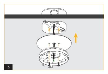
Use two Phillips screws to secure the canopy to the crossbar, going through the cover plate.
