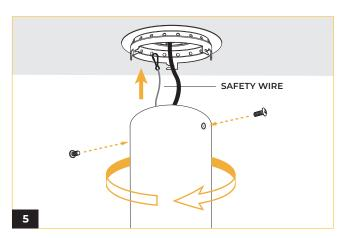
Attach the safety wires to the fixture lid. Secure the fixture and secure it using two Allen screws.
