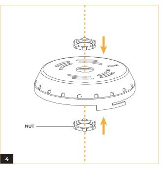
Screw lid to powerfeed tube with one nut on each side of the lid. Attach cylinder fixture to lid and secure allen screws.
