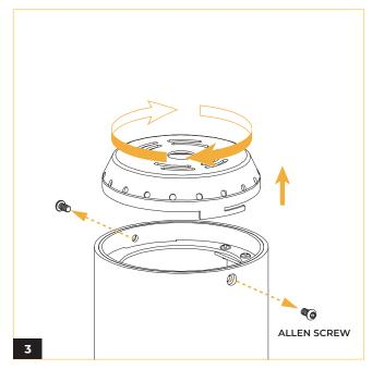
Loosen two allen screws on the side of fixture. Twist and remove the lid from cylinder fixture.
