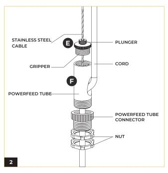
**(E)** Insert the cable through the gripper and plunger. Trim off extra cable using cable cutting tool. To adjust the cable to desired length, press the plunger.
