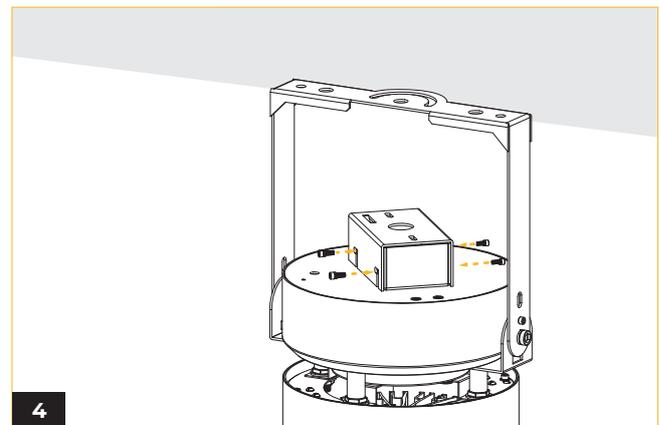
Screw 4 phillips screws to secure the wiring box.
