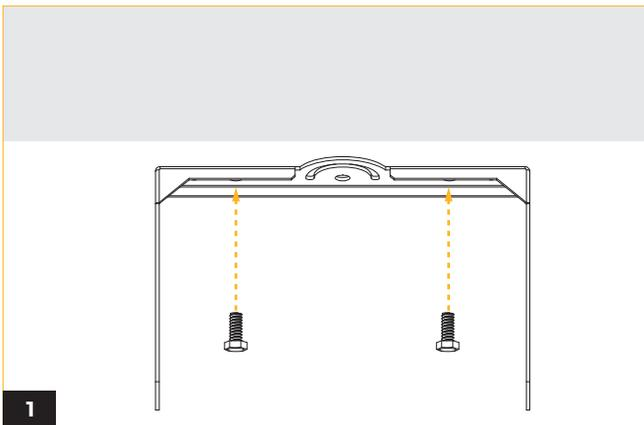
Secure Yoke Mount to surface with mounting hardware (by others) that is sufficient to support the weight of the fixture.
