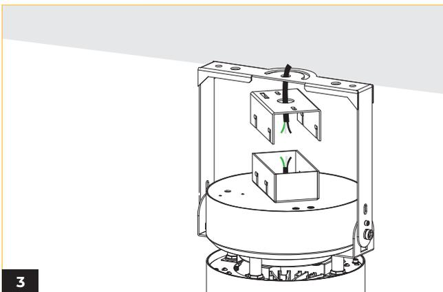
Connect electrical wires, refer to the wiring diagram for more information.
