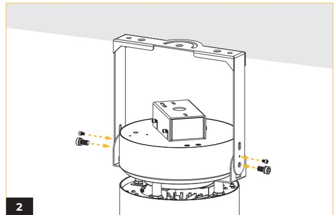
Loosen four Phillips screws on the side of the wiring box to remove the mounting bracket.
