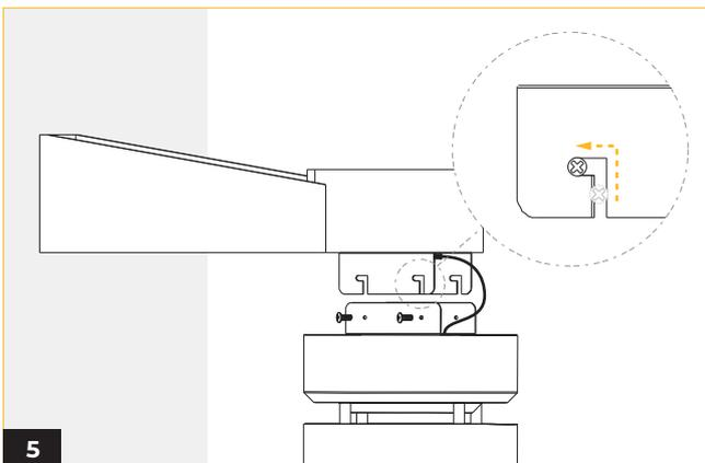
Screw 4 phillips screws to secure the wiring box on the mounting bracket. Lock and latch onto the mounting bracket, and tighten in place once secured.
