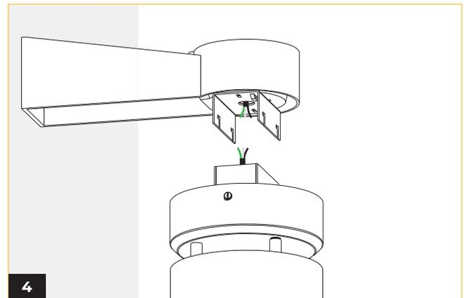
Connect electrical wires, refer to the wiring diagram for more information.
