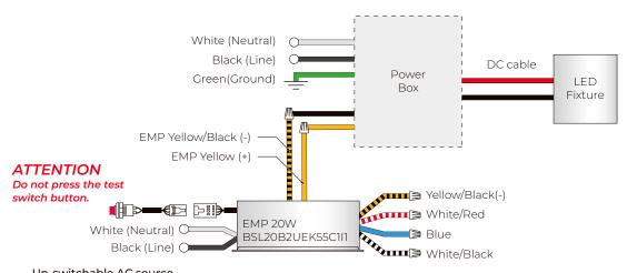
Un-switchable AC source To detect AC power outage
