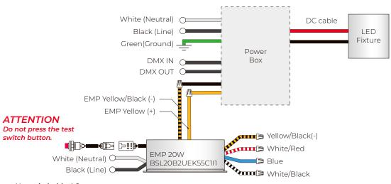
Un-switchable AC source To detect AC power outage
