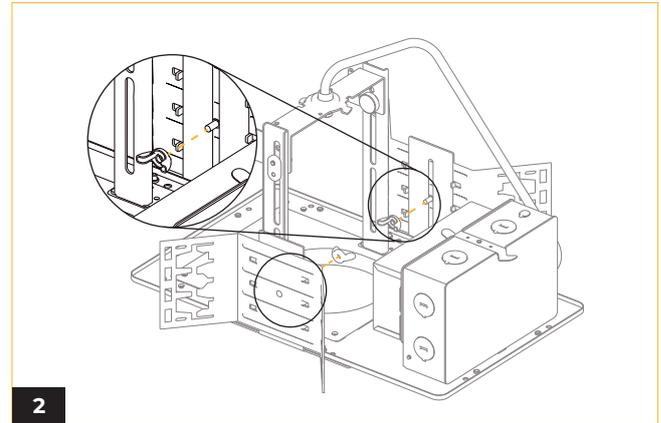
Secure the butterfly bracket by screwing in the provided wing nut.
