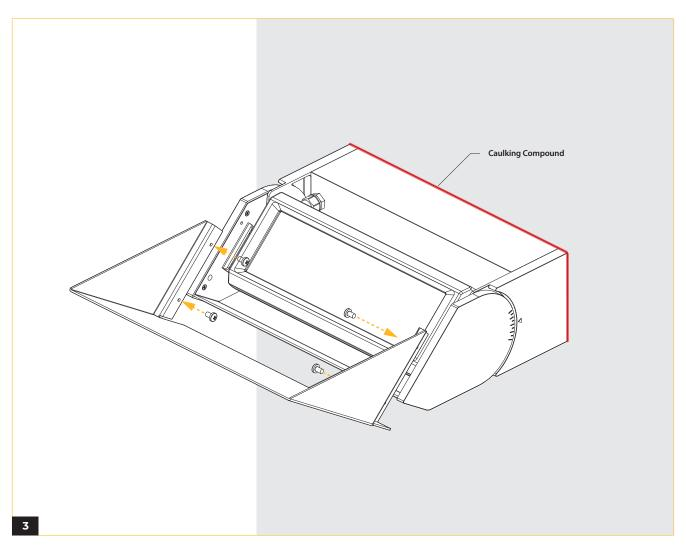
Apply caulking compound on the perimeter of luminaire if installed in an outdoor or natatorium setting. Install visor in front of lighthead if specified.
