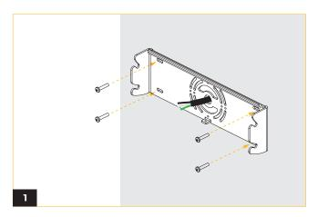
Thread wires through mounting plate and attach directly to wall. Use expansion screws (not provided) if mounting on concrete.
