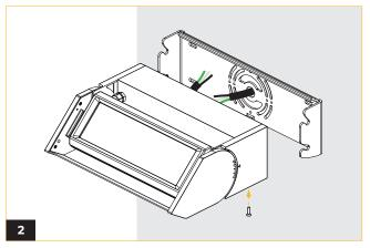
Hoist luminaire to the bracket and fasten from underneath.
