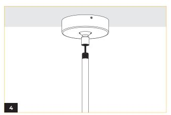
Thread the stem into the half ball, ensuring that the supply wires are passed through the stem.
