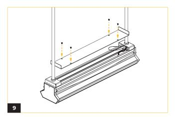
Replace the top cover and fasten it securely with the four screws.
