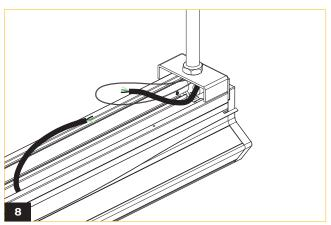
Pull the power wires through the stem and connect them to the fixture's internal wiring (refer to the wiring diagram).
