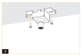
Mount the swivel crossbar onto a flat surface and secure it using the provided screws.
