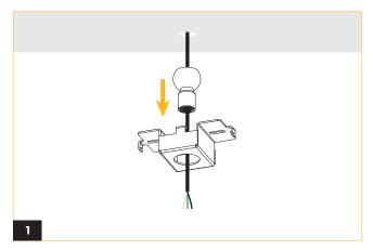
Insert the half ball through the opening in the swivel crossbar. Thread the AC wires through both the half ball and the swivel crossbar.
