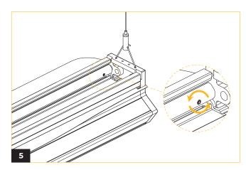
Ensure the blade angle aligns with the indicator, then secure it in place by fastening the screws from the inside.
