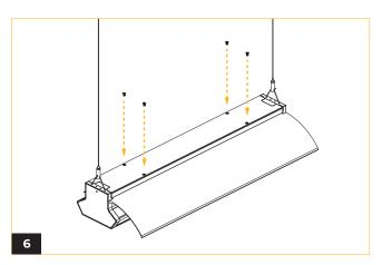
Reinstall the top cover by fastening the four screws.
