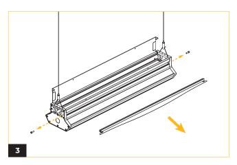
Loosen the mounting screws and carefully remove the diffuser. Handle with care to prevent scratches or damage.
