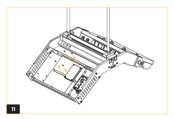
Unscrew the four screws to detach the lid of the waterproof junction box.
