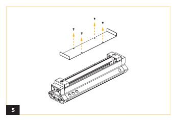
Remove the four screws from the top cover and carefully lift the cover upward.
