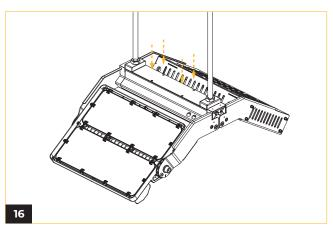
Replace the top cover and fasten it securely with the four screws. Do not overtighten.
