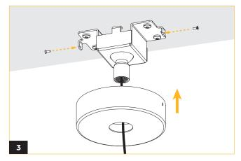
Position the canopy over the crossbar and fasten it firmly in place with screws on both sides.
