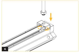
Position the stem against the mounting surface and secure it tightly using the lock nut.
