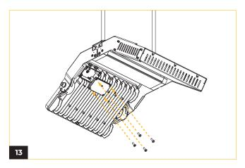
Reinstall the lid onto the waterproof junction box and fasten it with the four screws.
