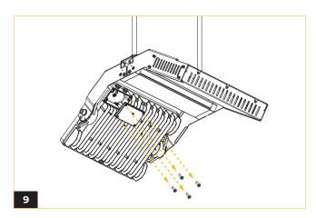
Loosen the screws and open the wiring access cover.
