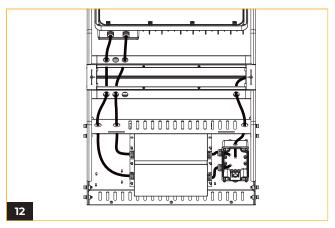
Thread the AC wire through the cable gland into the junction box. Establish electrical connections between the junction box and the fixture. (Refer to wiring diagram)
