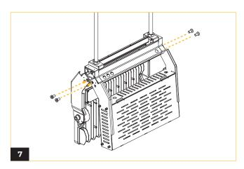
Align the luminaire body with the inner screw points. Fasten the fixture with two screws on each side. Ensure the body is securely fixed and stable.
