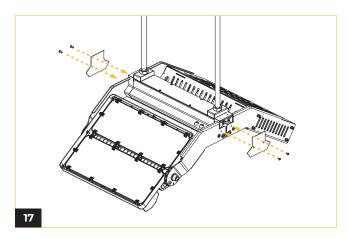
Install the cover plates on both the left and right sides to complete the assembly.
