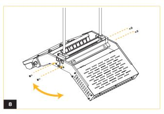
Extend the luminaire body until the outer screw points are aligned. Fasten the fixture with two screws on each side. Verify that the body is securely fixed and remains stable.
