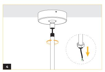
Thread the stem into the half ball, ensuring that the supply wires are passed through the stem.
