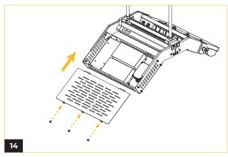
Reattach the power box cover by securing it with the three screws on the bottom.
