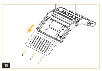
Remove the three screws located on the bottom to gain access to the power box.
