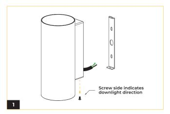
Remove the bottom screw and detach mounting plate from cylinder.
