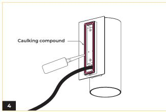
Apply silicone-based caulking compound along the perimeter of the mounting plate.
