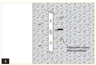
Attach mounting plate directly to wall. Use expansion screws (Not provided) if mounting on concrete.
