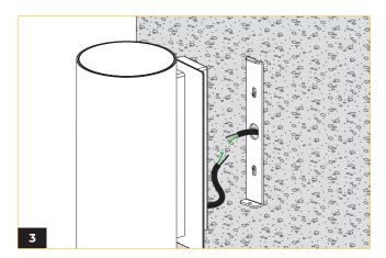
Slide in the cover plate to the cylinder and make electrial connections depending on dimming type (see wiring diagram).
