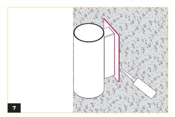
Slide the cover plate onto the surface, and apply one last silicone-based caulking compound along the perimeter of the fixture grooves.
