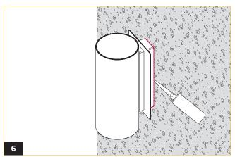
Apply silicone-based caulking compound along the perimeter of the wall mount bracket.
