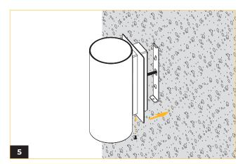
Attach cylinder fixture to mounting plate and secure by tightening the bottom screw.
