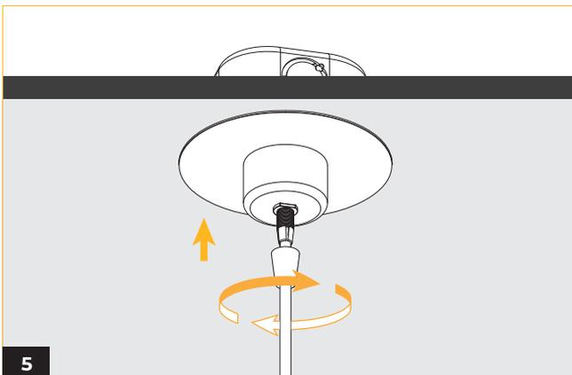
5 Screw in the cord grip cap to finish the installation.
