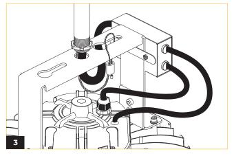
Clasp safety cable onto allocated slots on fixture bracket mount.
