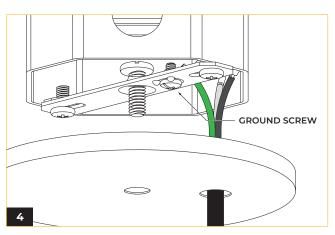
Connect the ground conductor to the ground screw on the crossbar, then connect the line and neutral wires according to the wiring diagram.
