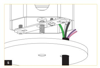
For 0-10V dimming option, connect the two remaining conductors according to the wiring diagram.
