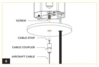
Thread the aircraft cable through the coupler with the terminal side on top. Slide the coupler up to the canopy and secure in place to the crossbar.
