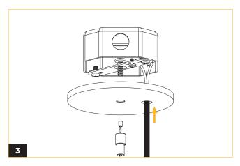
Thread the power cord and dimming wires through the canopy wire hole.
