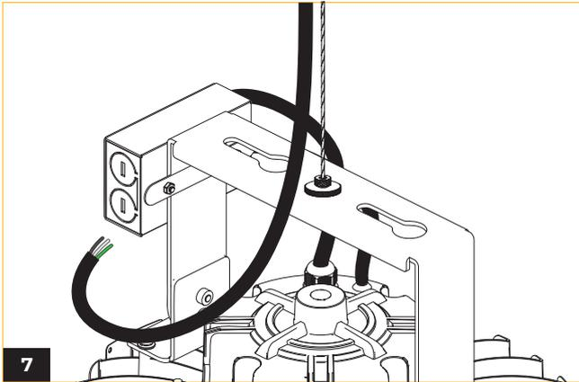
Make electric connection in junction box according to the wiring diagram.
