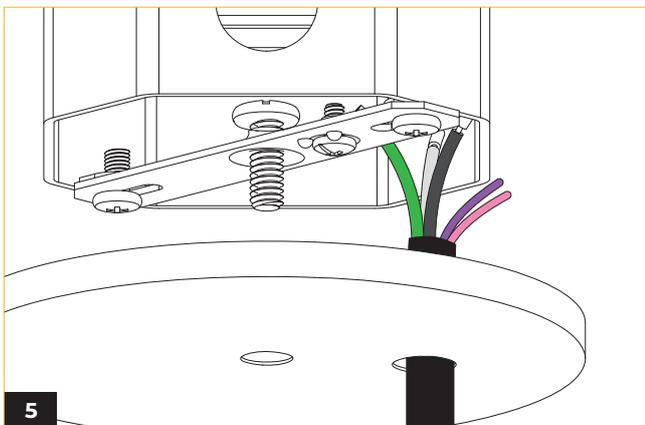
5 For 0-10V dimming option, connect the two remaining conductors according to the wiring diagram.
