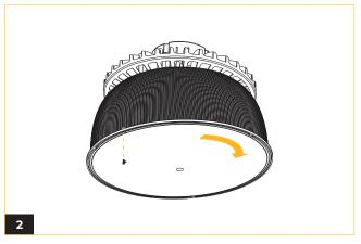
Push the cover in a clockwise direction to make the clips locked tight, and fasten the PC shroud and conical lens with the supplied screw.
