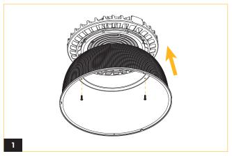
Install the PC shroud to the fixture with 3 supplied screws.
