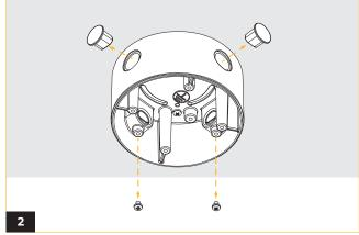
Remove the screws from the bottom of the junction box to release the conduit end caps.
