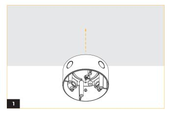
Attach the conduit mount junction box to the desired ceiling position by using mounting hardware. Ensure that the conduit openings are oriented in the desired direction.
