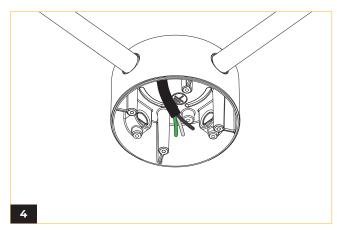
Thread the wires through the conduits.
