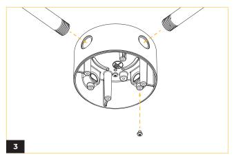
Attach the conduit to the junction box. If the conduit has threads, screw it in firmly. If the conduit is threadless, reattach the screw from below to firmly secure the conduit in place.
