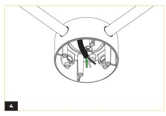
Thread the wires through the conduits.
