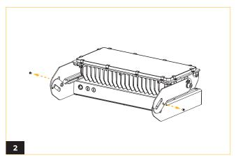
Unscrew the 2 outer fixed screws from the bracket.
