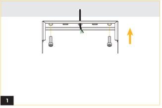
Secure the mounting bracket to a level surface using appropriate mounting hardware capable of supporting the fixture's weight. (350W: 24.25 lbs)
