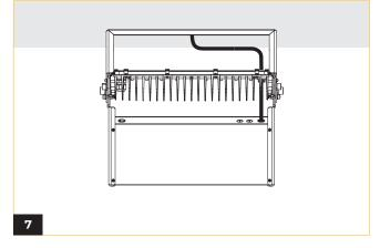
Establish electrical connections between the junction box and the fixture. (Refer to wiring diagram)
