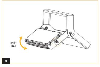
The light engine can be adjusted within a range of  $\pm 45$  degrees. To secure the rotated position, tighten the screws on each side.
