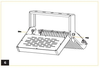
Secure the bracket by screwing back the two outer fixed screws.
