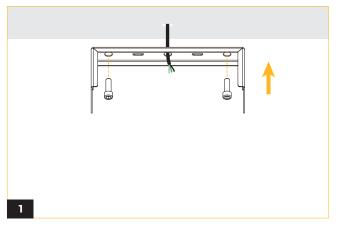
Secure the mounting bracket to a level surface using appropriate mounting hardware capable of supporting the fixture's weight. (700W: 44 lbs, 1050W: 77 lbs)
