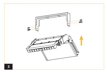
Align the bracket with the luminaire body, and fasten the bracket by using two screws on each side. Ensure that the unfolded body is also securely fixed and remains stable.
