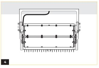
Establish electrical connections between the junction box and the fixture. (Refer to wiring diagram)
