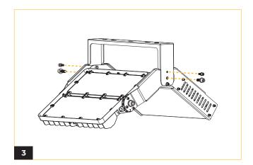
Fasten the bracket by using two screws on each side. Ensure that the unfolded body is also securely fixed and remains stable.
