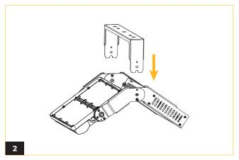
Align the bracket with the luminaire body.
