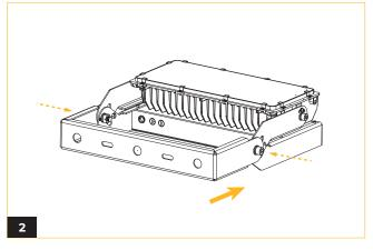
Align the bracket with the luminaire body. Fasten the bracket by using two screws on each side.
