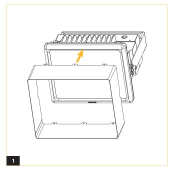
Put the shield on the fixture. Align the shield to the top of the fixture so the screw holes line up.
