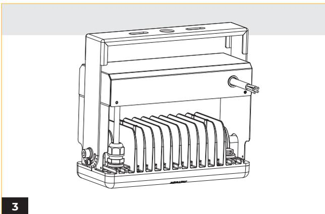
Establish electrical connections (Refer to wiring diagram)
