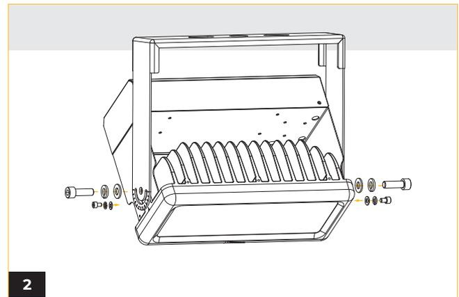
Slip the power box hook with fastener over the lock-in grooves allocated and fasten screws on either side to keep the power box in place.
