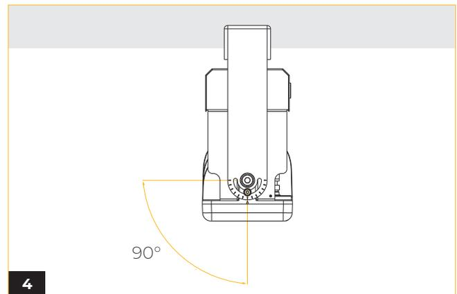
The light engine can be adjusted within a range of  $\pm 90$  degrees. To secure the rotated position, tighten the screws on each side.
