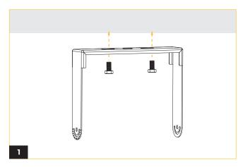
Secure bracket to a level surface with mounting hardware that is sufficient to support weight of the fixture and power box
