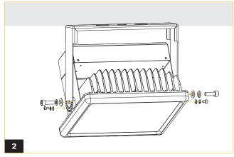
Slip the power box hook with fastener over the lock-in grooves allocated and fasten screws on either side to keep the power box in place.
