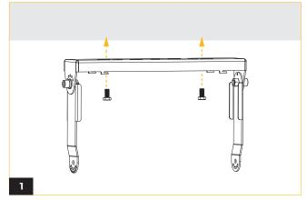
Secure bracket to a level surface with mounting hardware that is sufficient to support weight of the fixture and power box.
