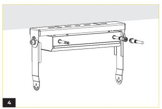
Connect quick connector cables between power box and fixture. Making sure to connect the AC wires(refer to wiring diagram).
