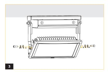
Secure the fixture to the bracket with provided screws.
