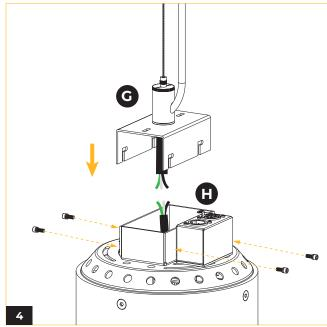
(G) Make electric connection inside the wiring box.
