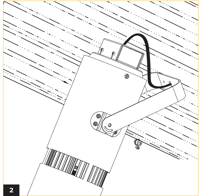
Route the wiring through the hole clearance on the bracket, and then fasten the fixture securely in place by tightening the screws.
