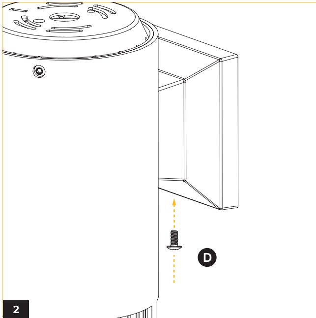
Secure fixture to mounting plate by locking the hex screw from underneath.
