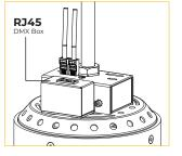
Connect DMX by using a standard shielded CAT  $\frac{5}{6}$  cable.
