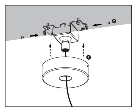
Step 3 Mount canopy onto mounting plate and lock in place with canopy set screws.
