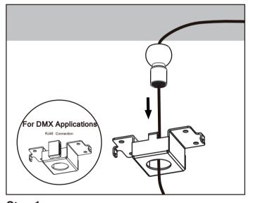
Step 1 Thread AC wires through swivel ball and mounting plate.
