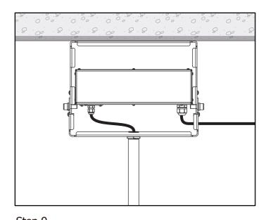
Step 9 Connect AC Cable to Junction Box.
