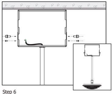
Align both lower and upper brackets and fasten in place.
