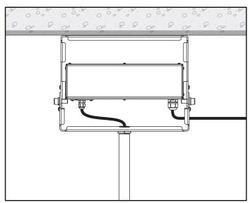
Step 10 Connect AC Cable to Junction Box.
