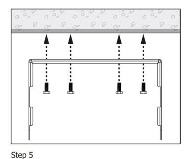
Fasten the top bracket on the desired location on the ceiling.
