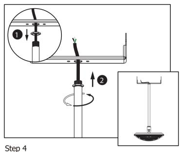
First, push the cables through a Hex screw and tighten on stem grooves. Second, fasten the stem onto the lower bracket.
