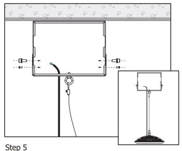
Align both lower and upper brackets and fasten in place.
