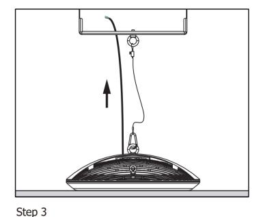
Attach the fixture cables through the lower bracket.
