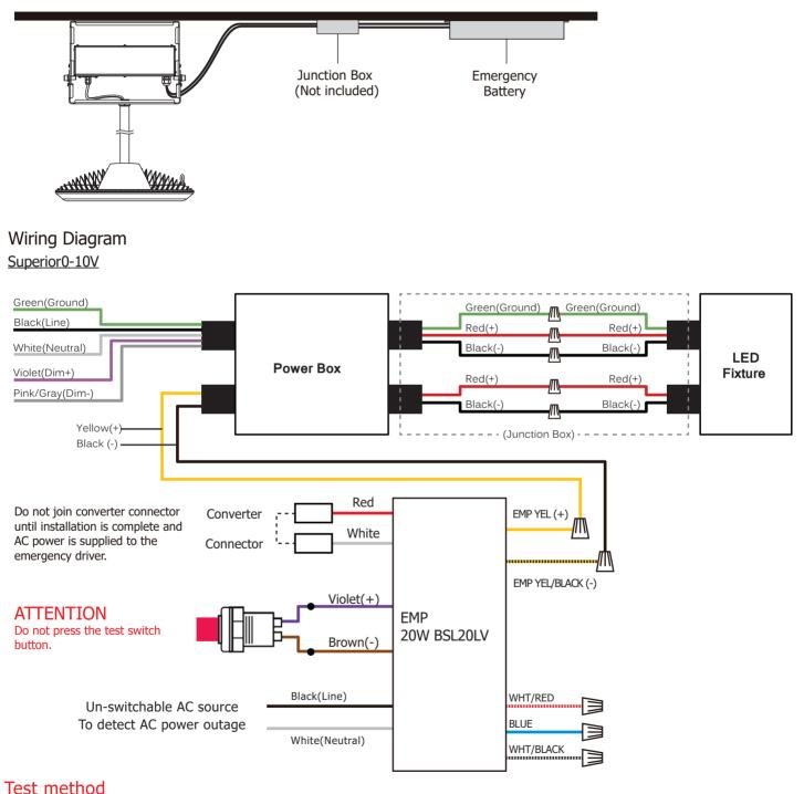
Disconnect the AC power of the LED fixture and EMP. The LED Fixture should be lit by EMP.
