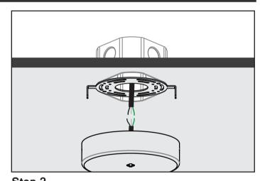
Step 2 Make electrical connections between junction box and fixture (refer to wiring diagram).
