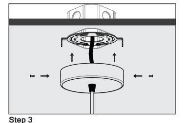
Cover junction box with mounting plate by securing 2 allen screws on either side of canopy.
