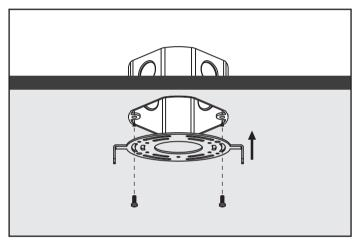
Step 1 Screw in the cord mount bracket on the junction box using 2 screws.
