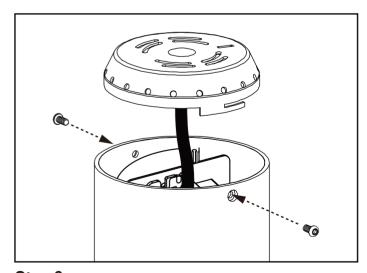
Step 9 Secure stem mount on fixture lid, and secure using two Allen screws.
