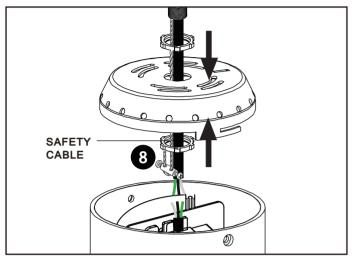
Step 8 Fasten nuts on both sides of fixture lid, and secure safety cables. Make electric connections inside the fixture (Refer to wiring diagram).
