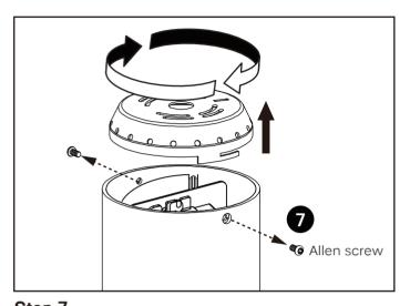
Step 7 Loosen two Allen screws. Twist and remove the lid from fixture.
