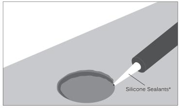
**Step 3** Apply sealant along inside edge of hole.
