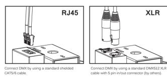
\*The last fixture has to be terminated with a DMX Terminator (by others).
