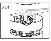
Connect DMX by using a standard shielded Connect DMX by using a standard CAT5/6 cable.
