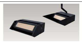
The REIZEN is an indirect asymmetric luminaire available in sconce or pendant forms, available with our Colorflip  $^{\text{TM}}$  W+RGB technology. 50% of the 150W Light Engine is true 3000K and 50% is RGB. This unique approach to RGBW color changing brings a multifaceted option to a variety of architectural high ceiling spaces such as commercial, education, hospitality, municipalities, retail, and sports-recreation areas.
