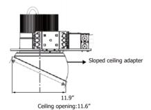
Cut 11.6" opening in ceiling for sloped ceiling adapter (same center as fixture frame opening)
