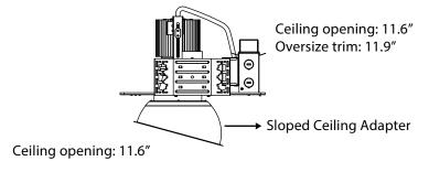
Cut 11.6" opening in ceiling for sloped ceiling adapter (same center as fixture frame opening)
