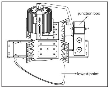
Align the fixture frame correctly on the slope ceiling adapter such that the junction box side is pointing towards the side where the slope is at the lowest point.
